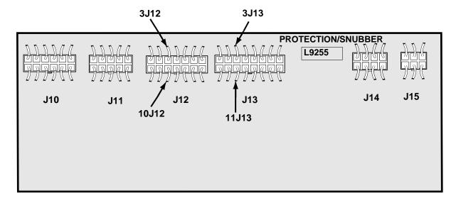
FIGURE F.9 - PROTECTION/SNUBBER BOARD TEST POINTS.
